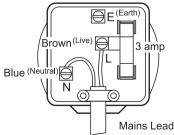
The wire coloured BLUE must be connected to the terminal marked N or coloured BLACK.
